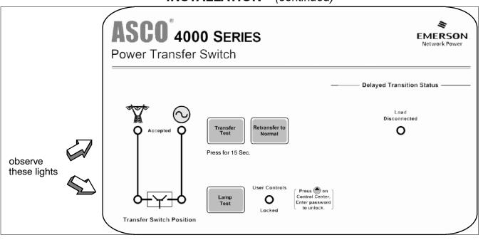
Figure 1-14. Standard controls and indicators.
